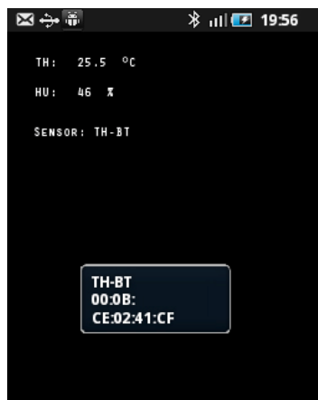
Fig. 3. The interface of the android-based application for acquiring environmental information via Bluetooth
