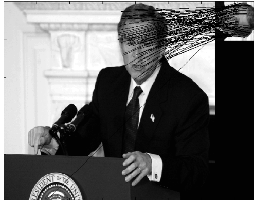
Fig. 2. Matched key-points in two different views of the same object (face)
