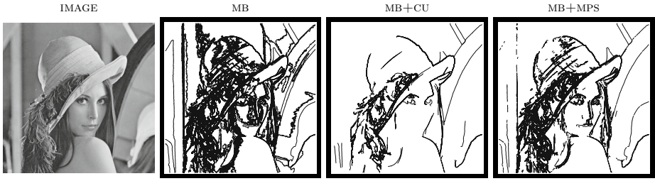
Fig. 2. Comparison of the results obtained with both clean-up algorithms. The one by Cao et al. (CU) [2] produces underdetection; this is corrected by using MPS.
