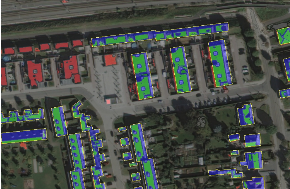
Fig. 2. Classified regions. Green for built regions mainly in building database polygon, Blue for polygon part not verified, Red for built regions not in the database.
