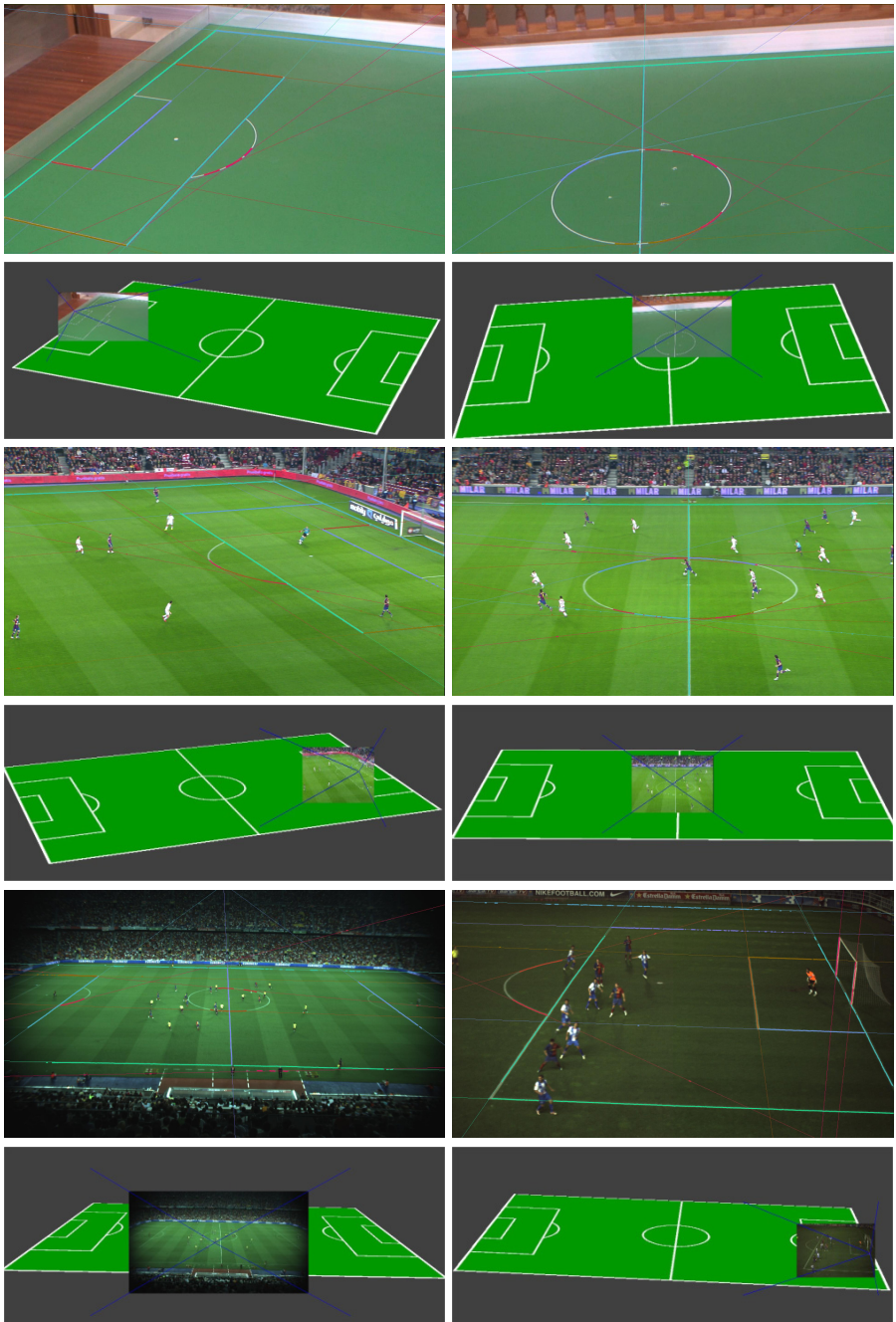
Fig. 2. Scale model and real images: Images on top are the detected lines. Bottom images are illustrations of the estimated pose of the camera in each top image.
