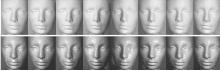
Fig. 4. Some sample images from the acquired databases. Top row: matte-painted styrofoam mannequin (for a Lambertian-like reflectance). Bottom row: styrofoam mannequin (for a specular-like reflectance). For both rows, variations along the x -axis are shown.
