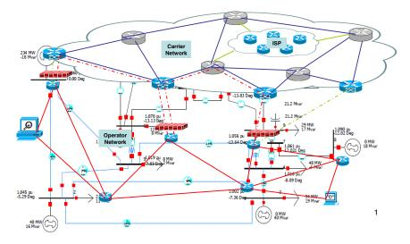
Fig. 4. SCADA system's interdependent ICT infrastructure
