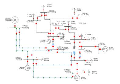
Fig. 2. The IEEE 14 bus test system
