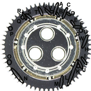
Fig. 4. Example of form collecting the labelled anomalies found on a ballbearing. The ballbearing is rejected as defective. The anomalies are evaluated with three intensities (1, 2 and 3), corresponding to levels of increasing seriousness of the anomaly (negligible, possible defect, serious defect).
