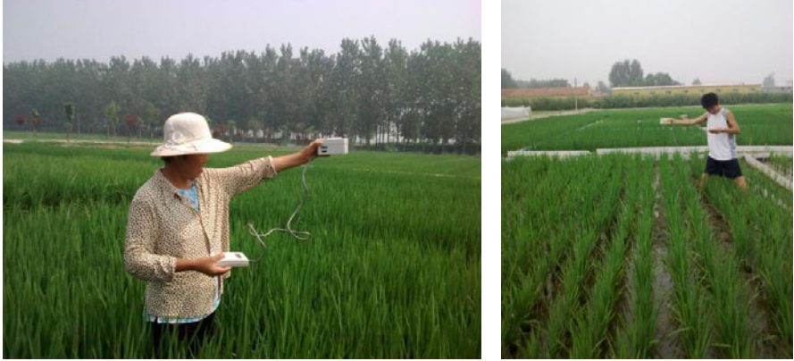
Fig. 4. RERI sensor used in field experiment. (In the 4th field experiment, handheld RERI sensor was used to measure rice canopy RERI values. The handheld RERI sensor was held 100 cm above the canopy under cloudless or partly cloudy conditions.)
