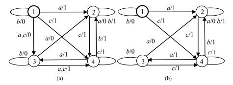
Fig. 1. (a) FSM 5 and (b) FSM B (initial states are in bold)
