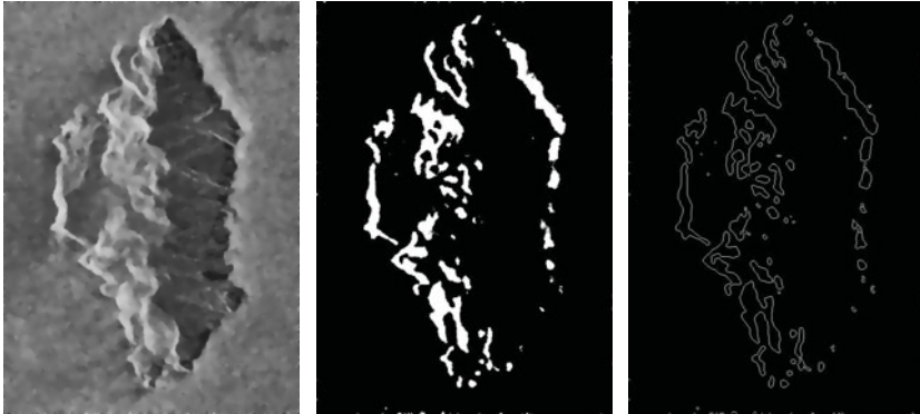
(a) Image of Capraia island smoothed by SRAD (b) Thresholding technique (c) Edge detection technique
