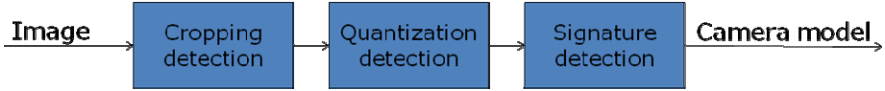
Fig. 1. Block based schema of the pipeline used to retrieve the camera model from an image
