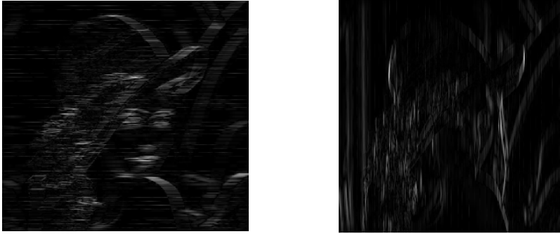
Fig. 7. 30 taps directional HPF applied to the Lena image. Borders are not considered (thus the vertical size in the left image and the horizontal size in the right images are less than the original size).
