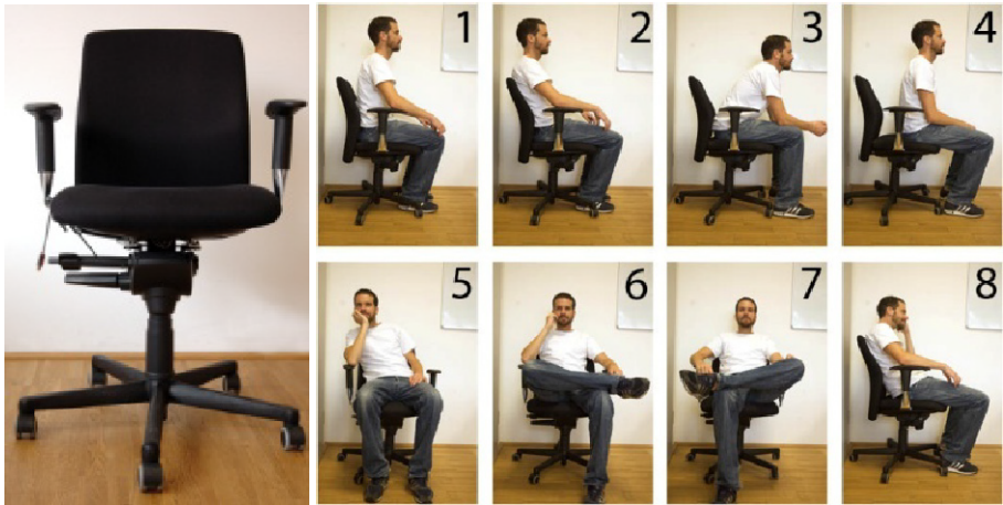
Fig. 1. Sitting postures that can be classified by the intelligent office chair. 1. upright, 2. leaning back, 3. leaning forward, 4. sitting at the front edge, 5. leaning right, 6. right leg crossed over left leg, 7. left leg crossed over right leg, 8. slouching.
