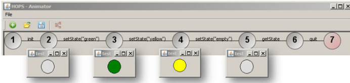
Fig. 7. The animation of operation sequence (init, setState(“green”), setState(“yellow”), setState(“empty”), getState, quit) controls the associated Java implementation of a peg hole
