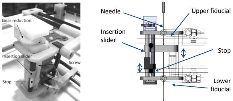
**Fig. 2.** Stop mechanism for setting the insertion stroke
