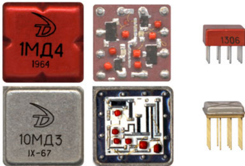
Fig. 7. First series IC in the USSR, “Tropa”, thick-film, a top number, “Posol”, thin-film, the bottom number. (At the left and in the center – in the double size, on the right – in full size).
