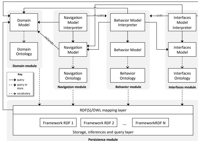
**Fig. 8.** Conceptual view of the Synth software architecture
