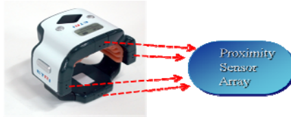
Fig. 3. Non-touch 3D space input mouse prototype: Armband-type
