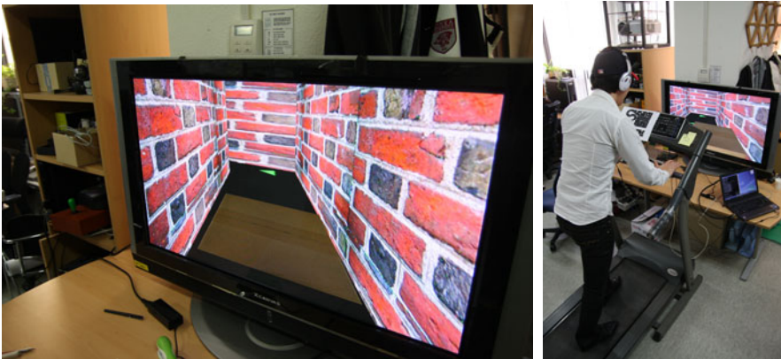
Fig. 3. A snapshot of the virtual maze used in the comparative experiment (left). A subject navigating the virtual maze using the interface set up. The G-Bar is installed on a heavy treadmill for grounding. The keyboard interface was also placed on the same place where the G-Bar was installed (right).
