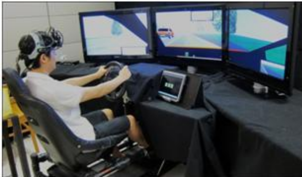
Fig. 1. The STISIM driving simulator and in-vehicle interface
