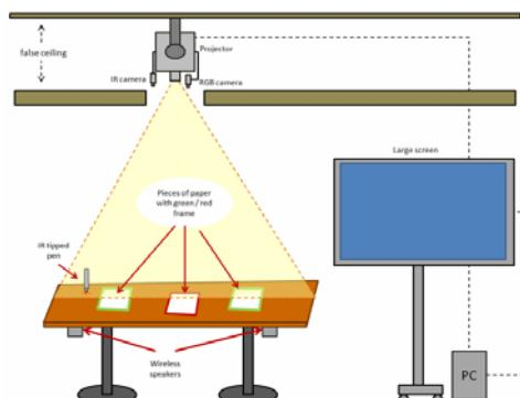
**Fig. 6.** PaperView schematic installation layout
