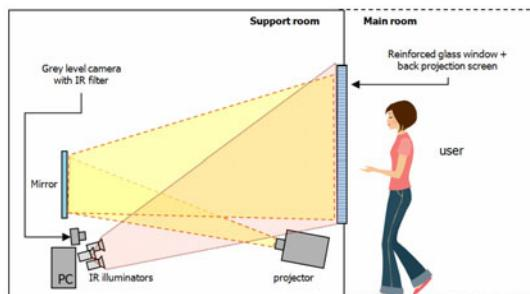
**Fig. 4.** Polyapton schematic installation layout
