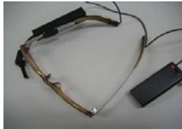
Fig. 4. Constantly wearable small see-through type HMD
