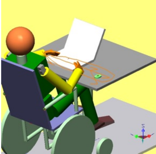
Fig. 3a. The anthropomorphic dynamic model represented in one specific position (see text). The track of the hand centre of mass during systematic analysis of the reaching is reported on the table by a orange line.
