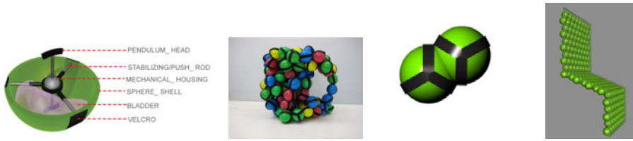
Fig. 5. This module used a pendulum-based spherical strategy for motion which adhered with Velcro
