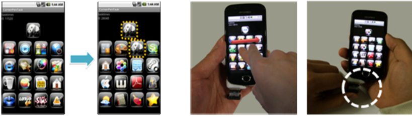
Fig. 4. The task of browsing (searching) and selecting an icon using the Finger-touch and CornerPen
