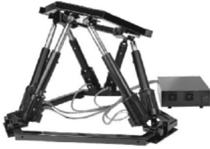
Fig. 8. Stewart platform for driving oscillation
