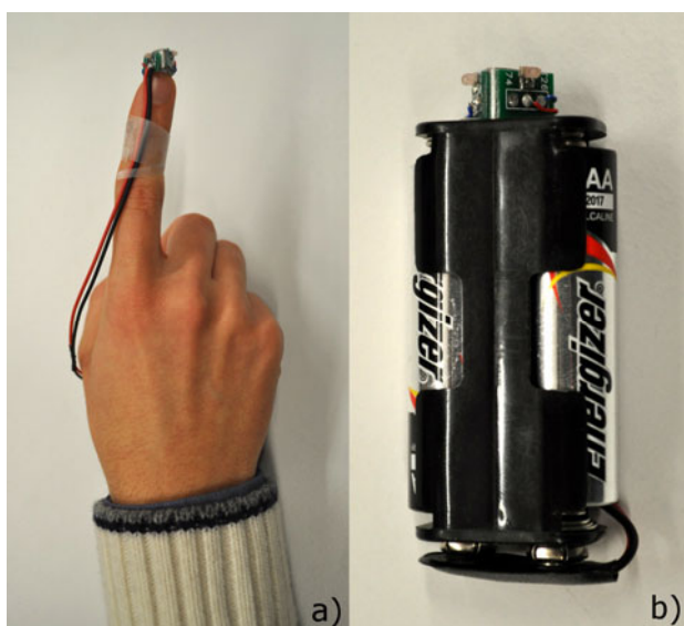
Fig. 2. Prototypes of the body worn infrared emitter ( left ) and of the handheld infrared emitter ( right )
