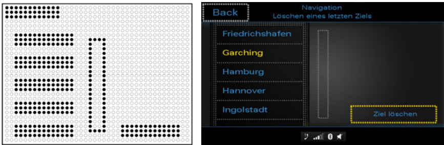
Fig. 4. Left: Elevated elements on the touchpad; Right: Displayed content on the middle screen with highlighted graphical widget
