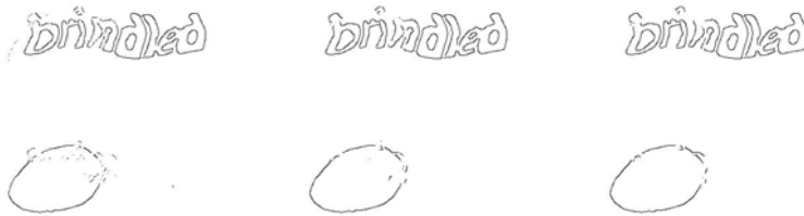
Fig. 4. Cascaded ellipse pixel classification. First row: pixels classified as “not ellipse,” second row: pixels classified as “ellipse.” From left to right: Classification after iteration 1, 4, and 9.
