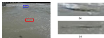
Fig. 2. An image with water wave and wood piece are highlighted, (b) upper portion of image is zoomed to show shape and color intensity of wave, (c) part of image is zoomed to show shape and color intensity of wood piece
