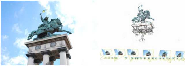
Fig. 4. The statue of Vercingetorix. The image set consists of 69 cameras. The algorithm creates 41274 tracks which are projected into 107078 image points, and 2869 of these are deemed outliers in the geometry estimation step.
