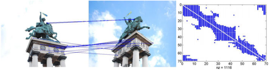
Fig. 2. Image nr 1 and 12 in the Vercingetorix sequence and matches when only matching the images directly. There are 20 matches (and it can be seen that at least two are incorrect). To the right is the adjacency matrix for the camera graph thresholded at 20 matches.
