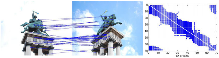
Fig. 3. Image nr 1 and 12 in the Vercingetorix sequence after running the tracking algorithm. There are 48 matches. To the right is the adjacency matrix for the camera graph thresholded at 20 matches.
