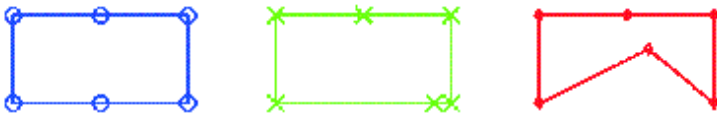
Fig. 6. Evaluation of the Segmentation: training shape (left), “correct” segmentation (mid, criterion A = 1, 0 ), and “incorrect” segmentation (right, criterion A = 0, 69 )
