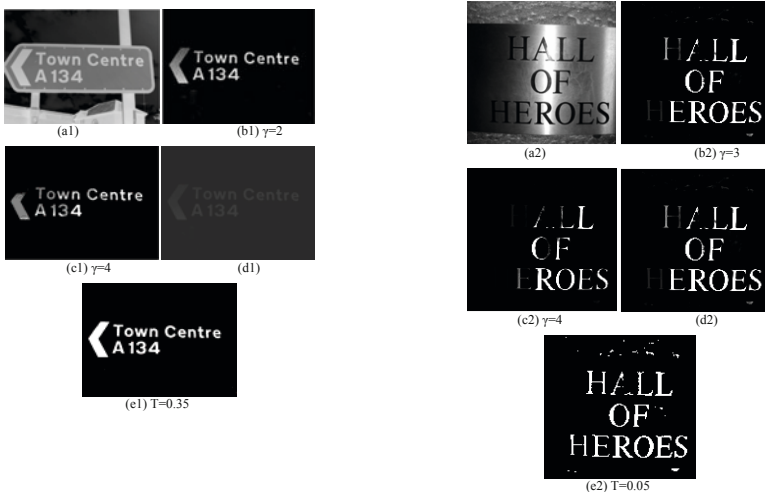
Fig. 6. (a) Original Images. (b) Gamma correction applied to connected opening (resp. closing) enhanced image. (c) Gamma correction applied to connected opening (resp. closing) enhanced image. (d) Difference between gamma corrected images. (e) Thresholded image.
