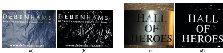
Fig. 9. (a) Input image with a complex background. (b) Threshold image. (c) Input image with over exposed background. (d) Threshold image.
