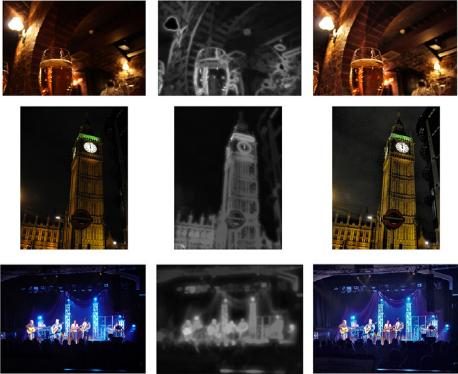
Fig. 6. Left: underexposed original images; middle: corresponding saliency maps; right: outputs of our whole method
