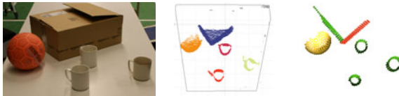
Fig. 8. Typical result of table, object, and shape detection. TOP: After fitting the planar model, the 20 753 inliers are removed and the table is represented solely by the model parameters and the convex hull of the inliers. The remaining 4591 points are segmented into 3 clusters (random colors) and successfully classified as being a sphere and two cylinders (see table below). The summarized results incl. ground truth information can be found in the table below. BOTTOM: Example of a more complex scene with one false detection (the left side of the box is detected as a cylinder due to the highly inaccurate data in this region). Colors are red (plane), green (cylinder) and yellow (sphere).
