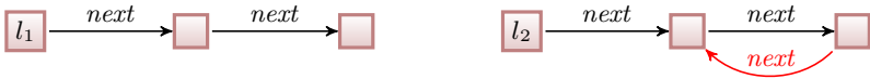
Fig. 5. Structures l_1 and l_2 are built with linked list nodes; l_2 is not acyclic
