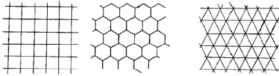
Fig. 1. Matrices used for pixel analysis. (a) Rectangular matrix. (b) Hexagonal matrix. (c) Triangular matrix.
