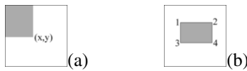
Fig. 4. Feature Estimation: (a) Integral image at point (x, y); (b) Four references to obtain the gray rectangular sum
