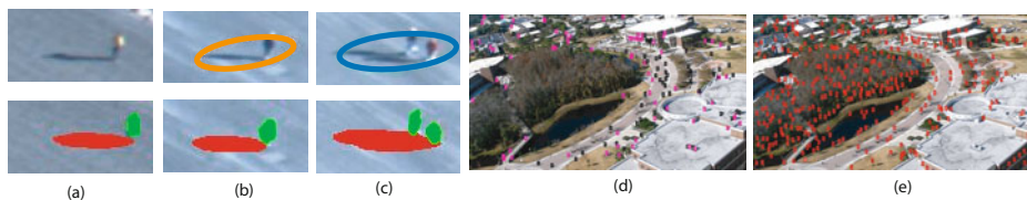
Fig. 8. (a) (b) and (c) compare motion detection (top row), and our geometry based method (bottom row). (a) Human is stationary and was not detected by the motion detector. (b) Moving blob includes shadow, the centroid of blob is not on the person. (c) Two moving blobs were merged by the tracker because of shadow overlap, centroid is not on either person. By contrast our method correctly detected and localized the human candidate (green). (d) and (e) compare geometry constrained human detection, and full frame HOG detection. Human candidates that were discarded by the wavelet classifier as clutter are shown in magenta , candidates that were classified as human are shown in black . Unconstrained full frame detection (e) generates many false positives.
