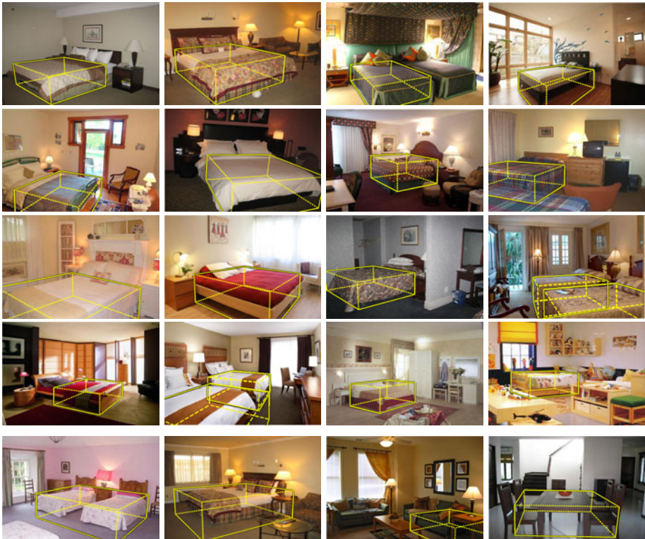
Fig. 5. Examples of high scoring detection selected from the first 100 top ranked detections of our algorithm on the test set images. First four rows show true positives, ground truth positive that are detected as positive and last row shows examples of false positives negatives that are detected as positives. Many false positives such as the the dining table and the sofa are due to high response of our detector to the strong oriented gradients in these areas.
