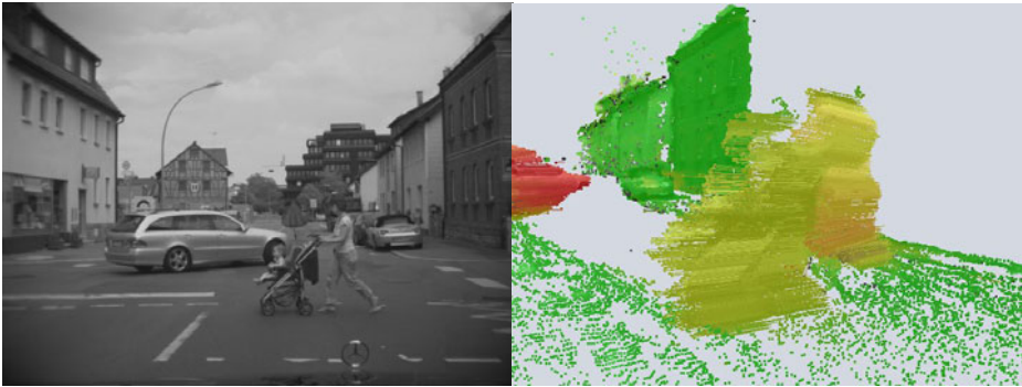
Fig. 1. left: typical traffic scene. right: motion field, estimated by the Dense6D algorithm proposed in this paper. The color encodes the velocity (from green to red) of the observed points.
