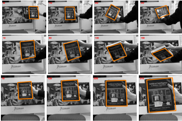
Fig. 2. Tracking through affine deformations. (row 1) Translation and subsequent rotation as the book rotates in plane over 90^\circ . (row 2) Shearing as book rotates significantly out-of-plane. (row 3) Scaling as book moves toward camera. Orange box indicates tracked target.
