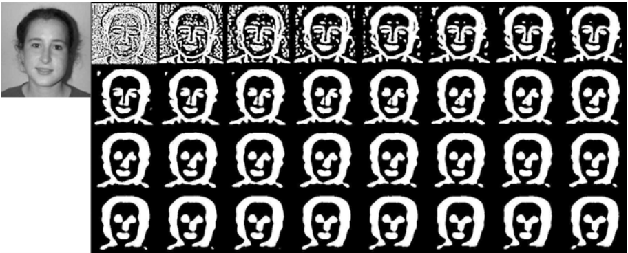
Fig. 1. The maximally convex regions \mathcal{L}_k > 0 are shown in white for k ranging from 1 to 100 in approximately equal steps. Image boundaries are handled in standard way: pad images by replication before processing, then remove boundary regions in the results. Unless otherwise indicated, input images in this paper are from Caltech 101 [7].
