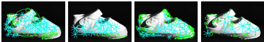
Fig. 9. Matching regular (green ellipses) and NF-features (cyan stars) of object 113 from the ALOI image database using NF-SIFT, NF-MSER, NF-HAff and NF-SURF
