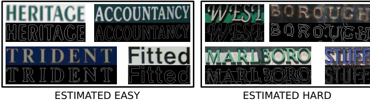
Fig. 6. In our analysis, we use a simple and intuitive heuristic based on edge detection to group images into EASY and HARD. The EASY examples are typically those whose characters are well outlined, and the HARD ones typically contain more broken characters and edges from the background and shadows. This is a coarse estimate of those images that are more CAPTCHA-like.
