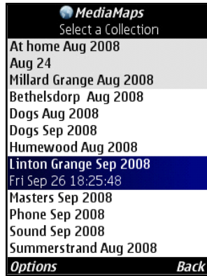
Fig. 3. Example of interface adaptation in MediaMaps, showing the adaptive section at the top of the list
