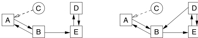
Fig. 5. Network layout after node C has switched to Mini mode (left) and after the resulting re-adaptation of node D (right)
