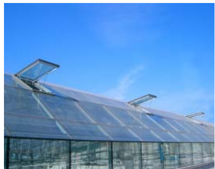
Fig. 6. The electrical rod actuators used in greenhouse window driving
