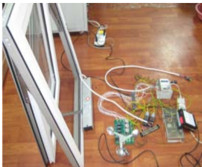
Fig. 5. Test of driving window with fuzzy control
