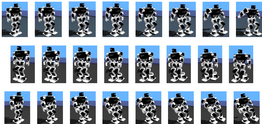
Fig. 3. Paths discovered by mRRT for left step forward ( top row ), left step backward ( middle row ) and left leg kick ( bottom row )
