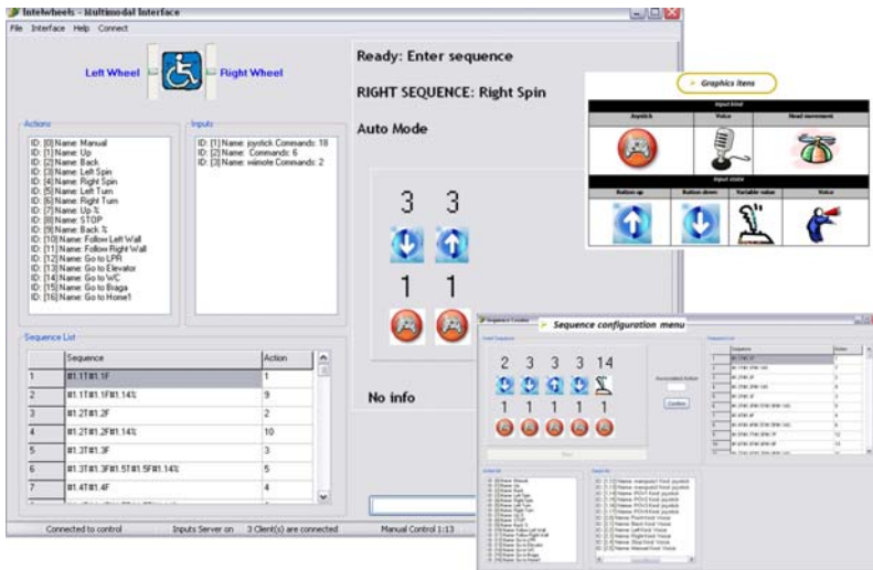
Fig. 5. Intelligent wheelchair multimodal interface design
